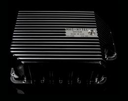
Deep sump, high capacity for maximum cooling. This pan increases fluid volume by (7) guarts. 1/8 NPT tap for temp. sender. Finned aircraft aluminum construction, drain plug with 303 stainless steel hardware. Increases case rigidity under hitorque conditions.
