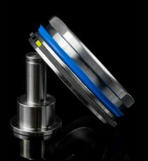
This newly designed piston is much wider and uses a teflon support ring along with lip seal to create a completely stable piston. This low/ reverse super servo is constructed from steel for strength and is available for 727 thru A518.
