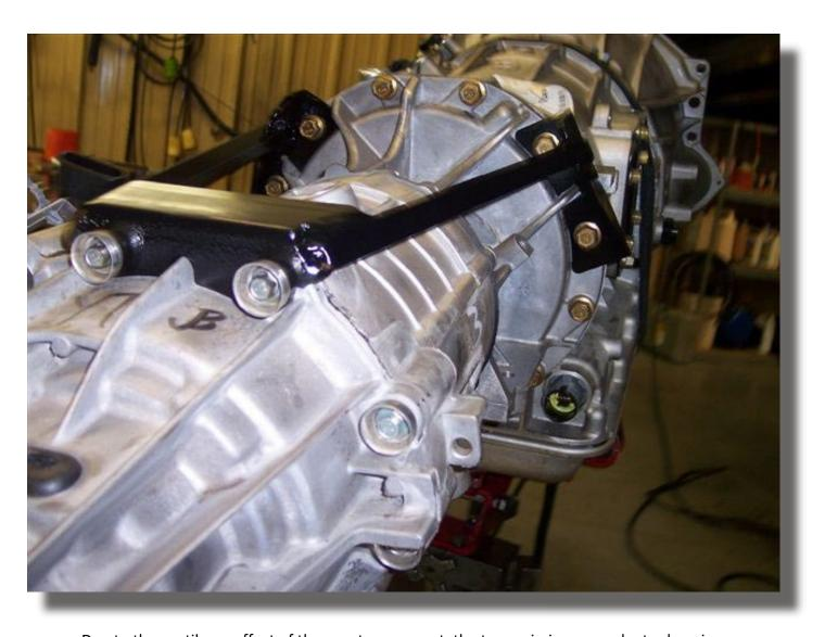
Due to the cantilever effect of the rear trans mount, the transmission rear adapter housing is prone to cracking. The slightest amount of rear drive shaft vibration can result in a very expensive transmission repair. Help your transmission with this easily installed brace. Installs in less than 30 minutes with no special modifications or tools required.
