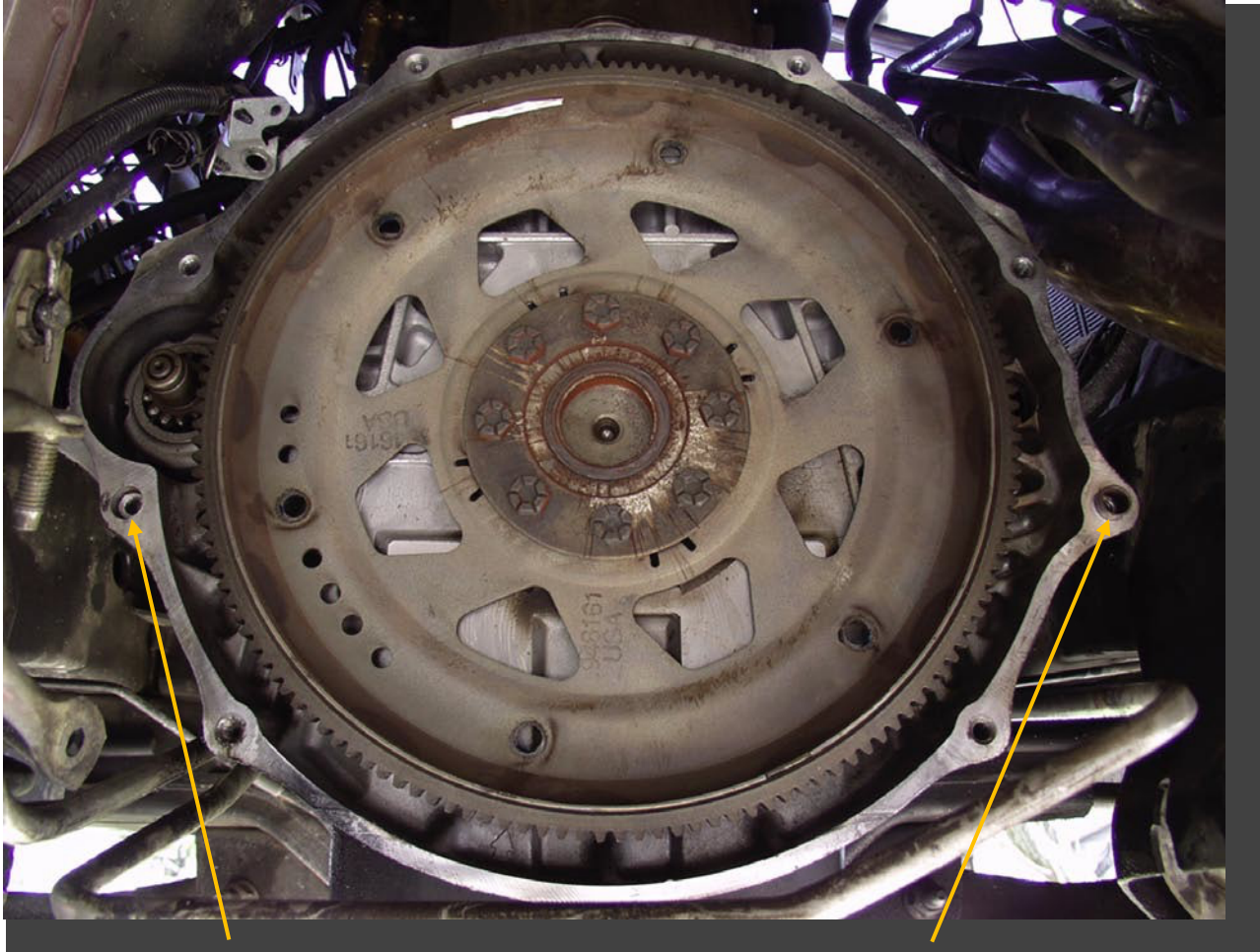
Dowel Pin Missing
