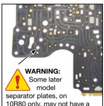
10R80 only, may not have a hole over the accumulator lineup. If there is no hole, it is not necessary to install this TCC signal damper piston kit.
