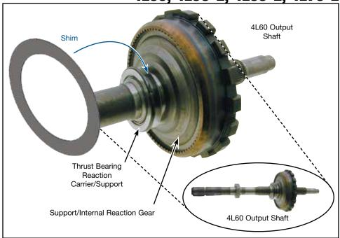
Use .010" thick Sonnax rear endplay shims between rear support and bearing to take up excess endplay clearance.
