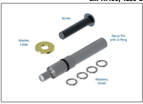
NOTE: If using an OE servo piston ('95-earlier 4L80-E or TH400), carefully inspect the aluminum casting for any indication of cracking. If the servo piston is damaged replace with Sonnax servo piston 34914-01. Target servo travel is .125". Determining the servo travel and required pin length can be accomplished several ways. The most common is to modify an extra servo cover to be used for setup before final assembly.
