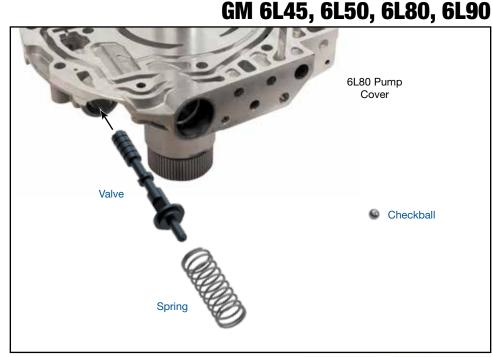
NOTE: In GM 6L45, 6L50, 6L80 and 6L90 units the pressure regulator valve and boost assembly are located in the pump cover. Transmission must be removed from the vehicle to access pump and replace the pressure regulator valve.
