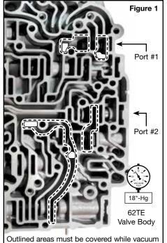
testing to receive results. Additionally, the holes highlighted within those areas must be plugged to receive results.
